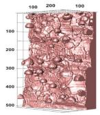
AM as-printed surfaces contain a multitude of features (image above) that can impact fatigue performance. VEXTEC incorporated the critical features as stress distributions (image below) and as distinct material layers in its VPS-MICRO modeling.
