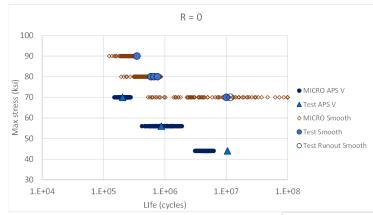
The VPS-MICRO model was first calibrated to R = 0 load ratio machined round bar fatigue specimens, then predictions were made for the fatigue knock-down due to APS (image above). The model was then extended to R = -1 load ratio (image right), and shows good agreement for predicting fatigue lives for APS knock-down and different load ratio.
