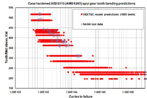
*This compares 21 test points, collected over the course of a year, with 10,000 virtual simulations produced using VLM in one-fourth the time. The "scatter" at each load point is indicative of real life processing variations expected in a fleet of parts. As shown, 21 physical test points can't adequately convey this.*
