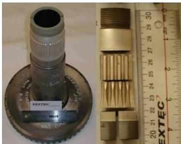
This is a photo of the gear shaft example. In order to properly simulate the processing grain arrangement complexities, the physical part was sectioned as shown. High resolution imaging is used to statistically evaluate these complexities during simulator preparation work.
