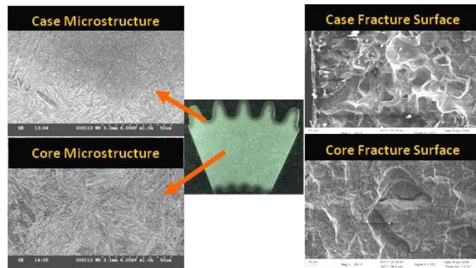
*Actual gear manufacturing creates a complexity of grain microstructure arrangements that are ignored by the standard AGMA modeling approach. As shown grain arrangement differentiations create variations in fracture mechanisms which are accurately reflected with VLM simulation results.*
